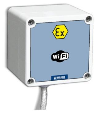
WIFI module for the wireless data communication in ATEX 2 and 22 zones, with protection methods according to: ATEX II 3G Ex nA IIB T6 Gc X for gases ATEX II 3D Ex tc IIIC T125°C Dc IP66 X for dust. It can be applied to both bench/floor scales as weel as mobile scales, such as pallet truck scales or pallet weighing scales. It allows the easy wireless connection to the company computer system and the data transmission at a very long distance.
